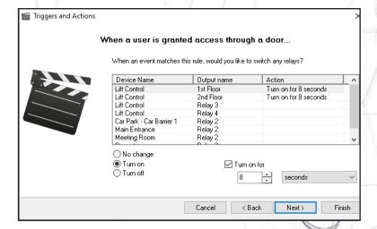
Set up a rule for each of the various floor button combinations as required.
