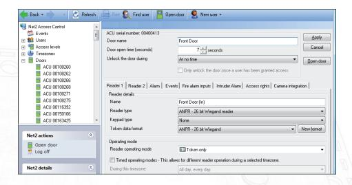
Run the Net2 software and select the ACU and reader port where the camera is connected.
