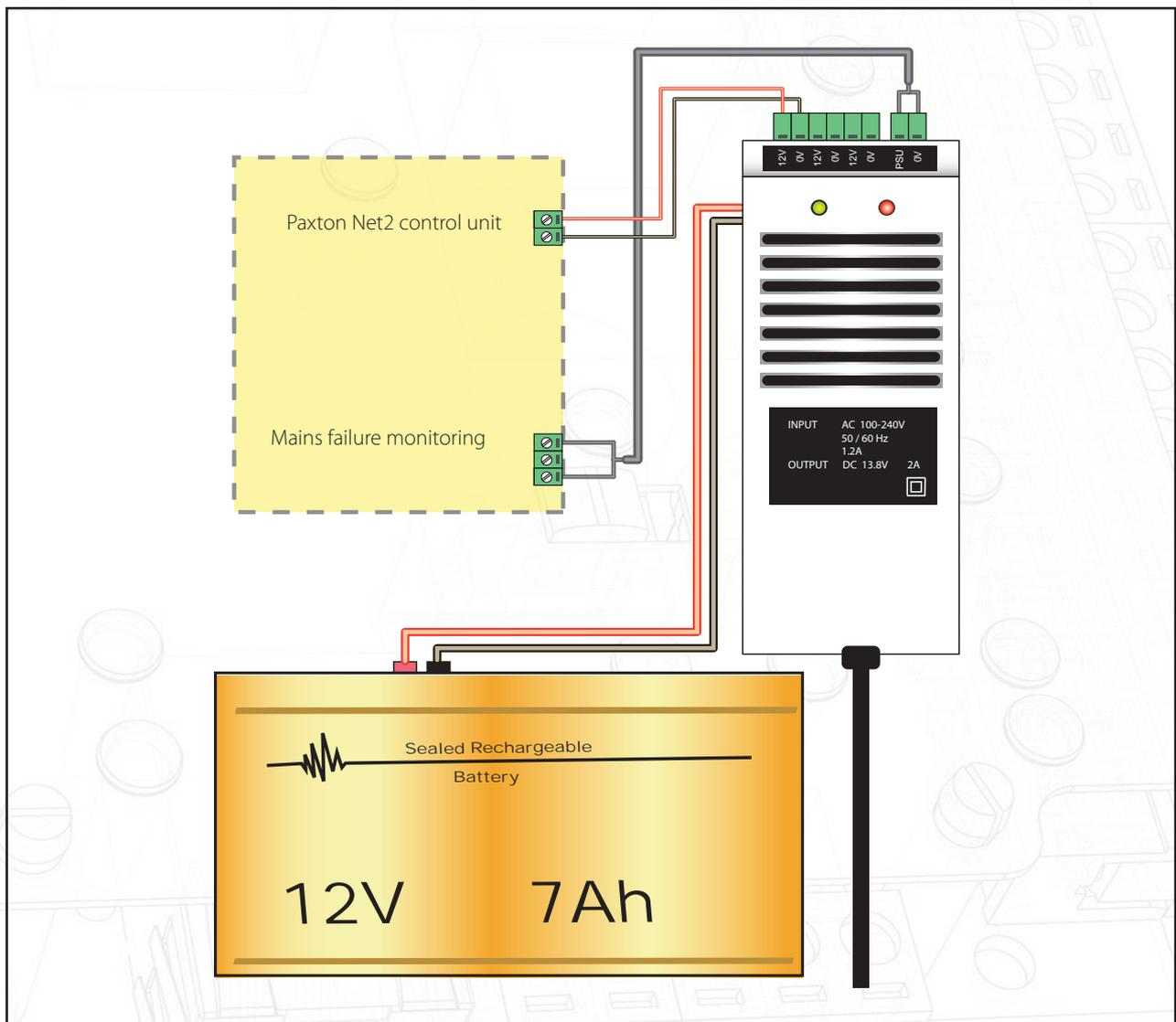
This ACU has an input for mains monitoring. This also requires the power supply to have a mains fail 'voltage free' relay output. The ACU will then report a mains fail alarm if this input changes state.
