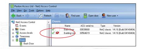
While the alarm output terminal on the ACU is active (held at 0V), an alarm icon is displayed against that ACU in the door display.
