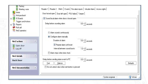
Each type of alarm has its own tab. The settings for each type can be different. (Net2 nano has fixed values)
