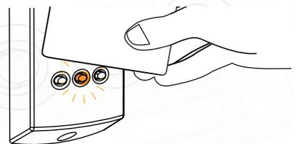
When presented to an inactivated HID™ reader and if the activation card has used all the licences available, the reader will emit a **red** LED to indicate the card is empty and another activation card should be purchased.
