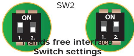
The hands free interface has a pair of switches labelled SW2. Select either switch 1 or 2 to set which button the interface will respond to and then power cycle the interface to store this setting.
