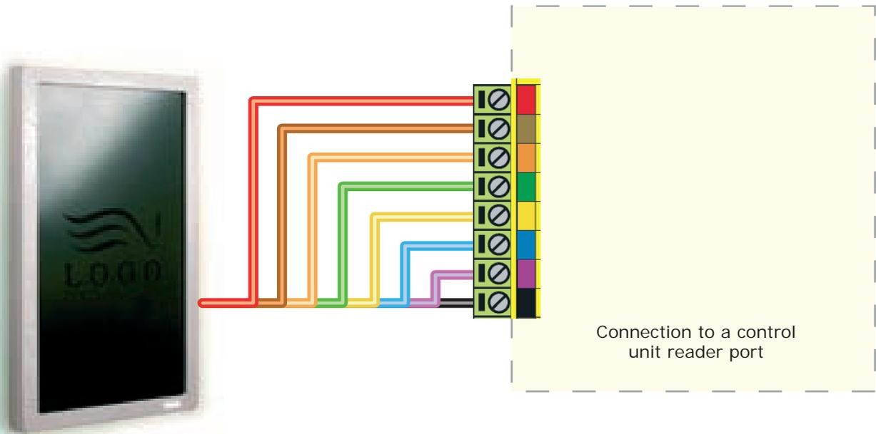
**IMPORTANT:** This reader cannot be connected in parallel with other readers and keypads.
