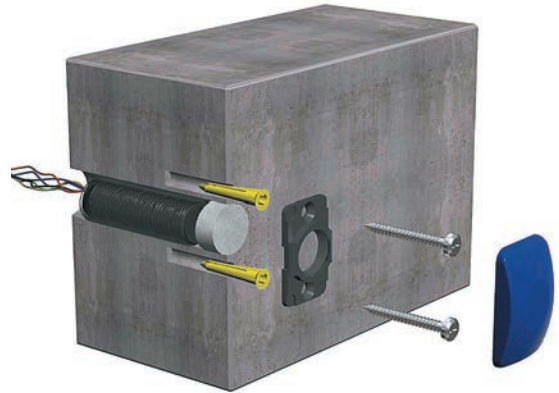
Cement plug - high vandal resistance
