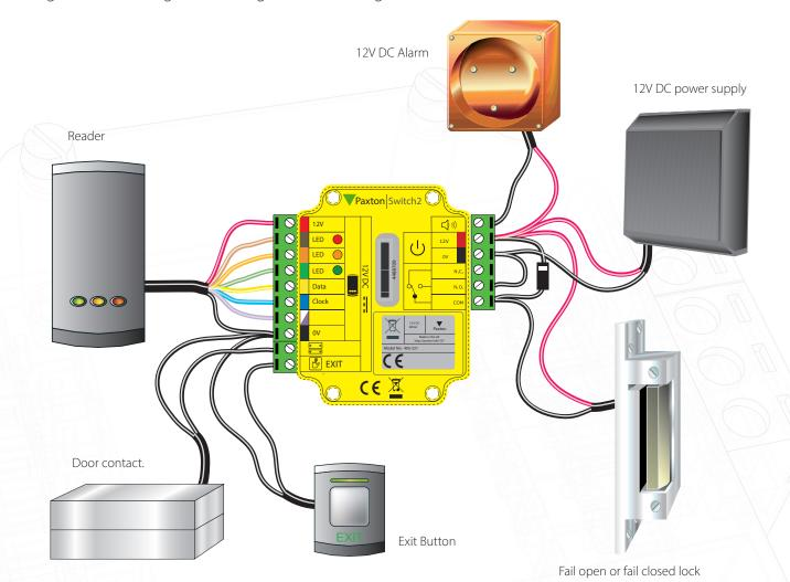
**Power connection** - the Switch2 control unit requires a 12V DC power supply connected to the "12V" and "0V" terminals. A simple 12V power supply with battery backup is recommended. The chosen supply must be capable of providing enough current to cope with the reader, the alarm sounder (if fitted) and whatever lock is connected to the system.
