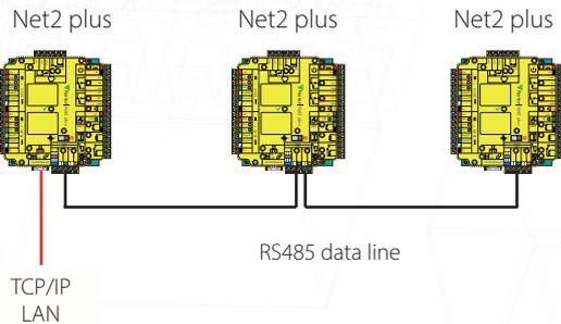
1 - The Net2 plus ACU's can be individually connected to the Net2 PC via the site LAN network.
