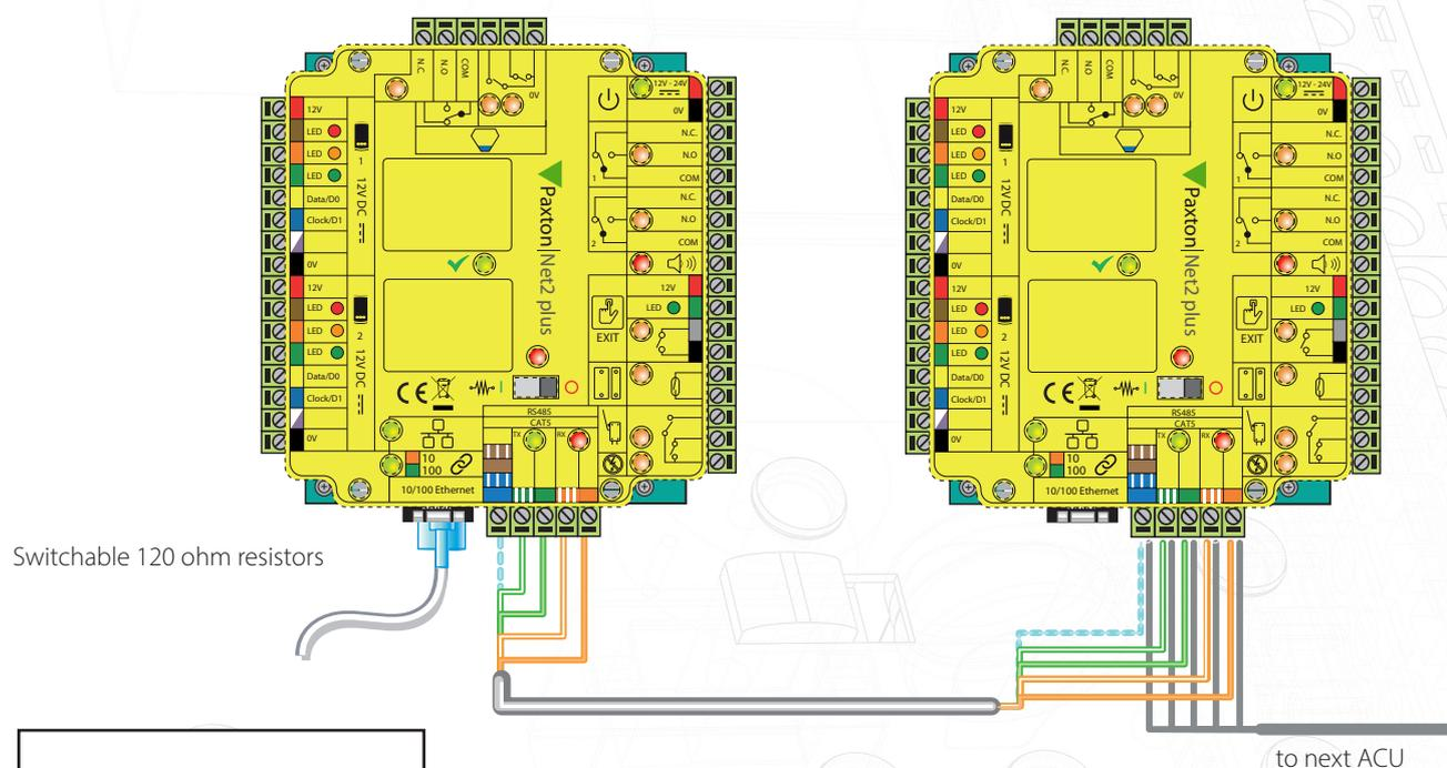
The Net2 plus plugs directly into the TCP/IP Ethernet network via a standard RJ45 connection box
