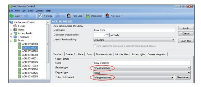
The filter information is stored in each ACU controller. Any changes to the Wiegand filter will require the Net2 server to be restarted so that it can update the system.
