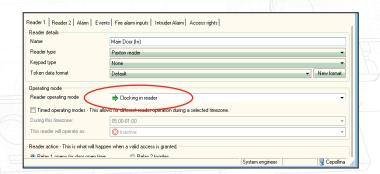
Dedicated readers are required for Clocking In and Clocking Out and cannot be used to control access through a door. Separating these functions ensures accurate time and attendance information.
