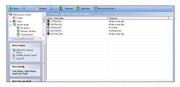
In the above example we see an entry in the table for every reader that has been enabled. The Car Park ACU has both In and Out readers installed and so this 4 door system has a total of 5 entries. Alongside each entry is the timezone that defines when this reader is active and users who are assigned this access level will use these reader restrictions.
