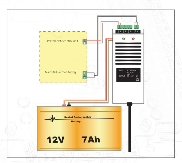
This ACU has an input for mains monitoring. This also requires the power supply to have a mains fail 'voltage free' relay output. The ACU will then report a mains fail alarm if this input changes state.
