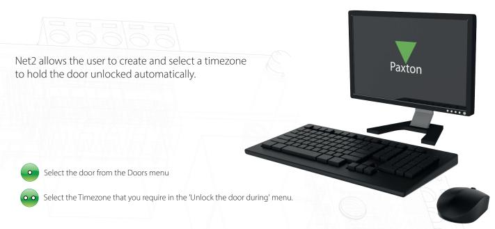
Under normal operation, this should be set to 'At no time' so that a valid user card must be presented each time to gain access.
