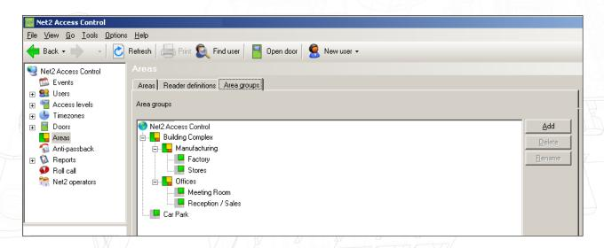
The same door must NOT be used to control two individual anti-passback boundaries.
