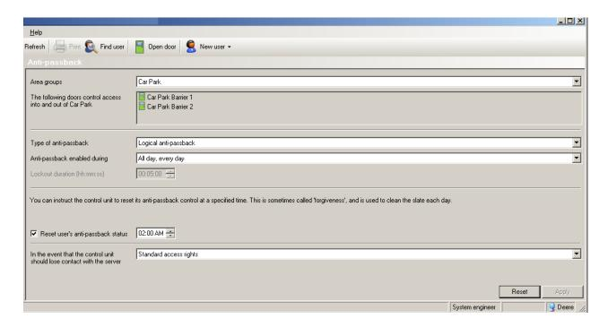
Anti-passback can be controlled by a time zone. This allows the system to be turned off when tight control is not required or desirable (e.g. out of hours).
