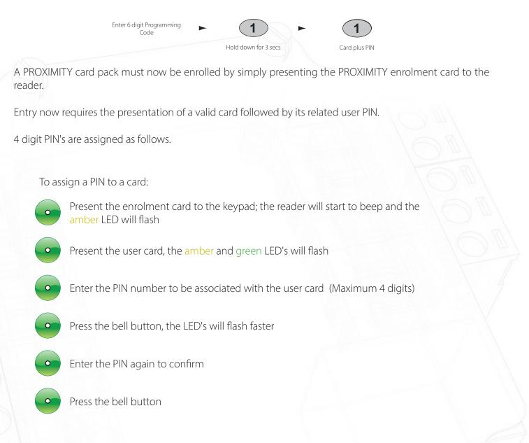
The user card and related PIN are now valid. When the user card is presented at the keypad the amber LED will light indicating that the keypad is waiting for the PIN. When the correct PIN is entered the door will open.
