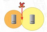
When using in and out readers, users may be picked up by both readers as they move through the door which will affect the reliability of any roll call or anti-passback application. Ensure that sufficient spacing is provided between these readers for optimum range and reliability.
