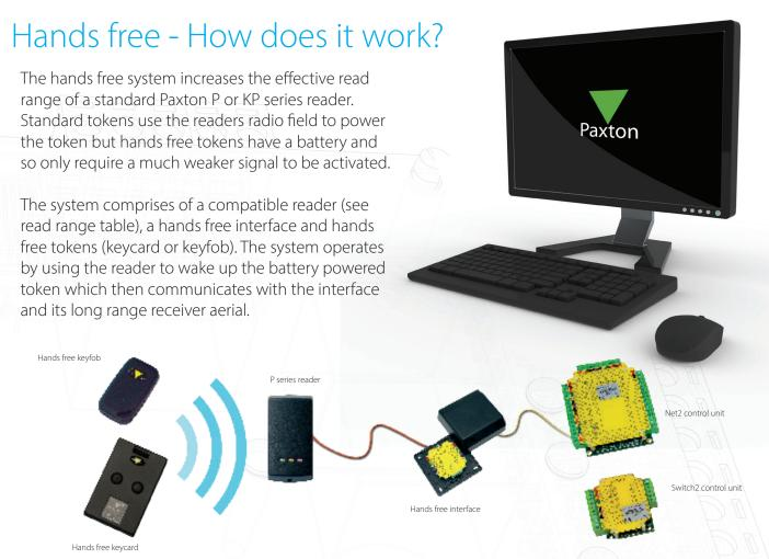
Existing P and KP readers can be used without modification. The hands free interface takes its power from the control unit and therefore does not require a power supply.
