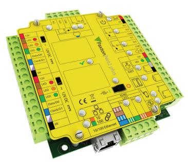
They can be used as part of the site LAN using the TCP/IP protocol. They are then connected to a Net2 plus or via a TCP/IP converter to run an RS485 data line for Net2 Classic units.
