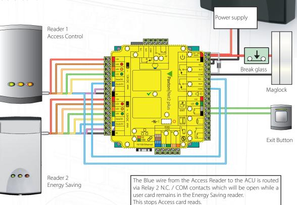
Wire the ACU as per a normal Maglock. As advised above, the 12V feed passes through an external break glass so that the lock can be released from the outside in an emergency.
