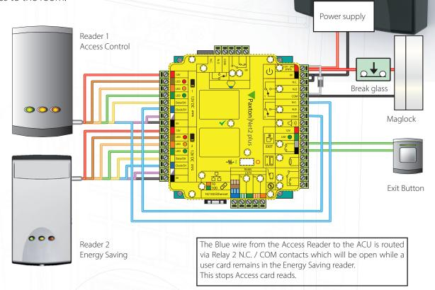
Wire the ACU as per a normal Maglock. As advised above, the 12V feed passes through an external break glass so that the lock can be released from the outside in an emergency.
