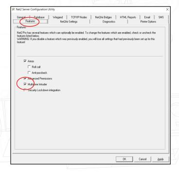
You must use Net2 Professional software v4.21 or later. Select the Features tab and check the Multizone Intruder box in the Server Configuration utility.
