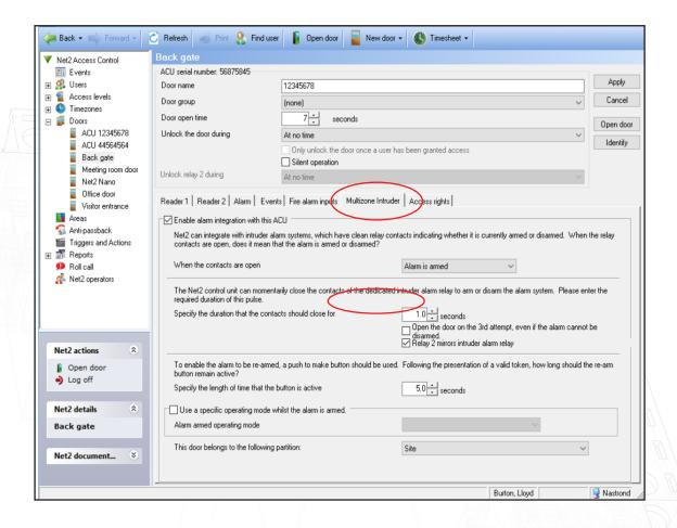
When Multizone intruder is enabled, the intruder alarm settings have an additional option to select the partition that the door relates to.
