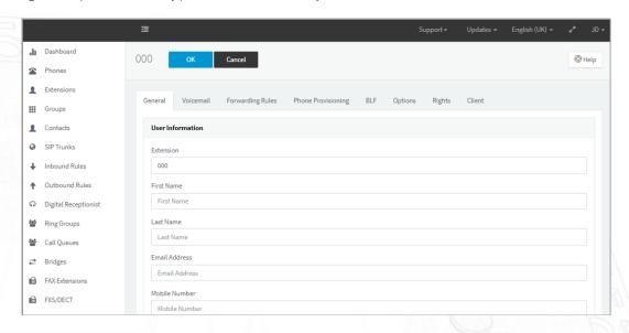
Create an Extension record for the panel. Set up an Extension number and add a Description as required in Name field. These can be any unused values.
