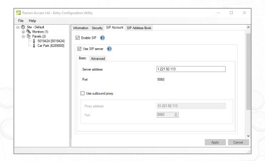
Within the Net2 Entry Configuration go to Site Settings - SIP Account tab and select 'Enable SIP Client' and 'Use SIP Server'
