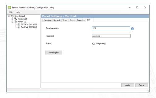
Then create a matching entry for the Panel within the Net2 Entry configuration, Panel Settings - SIP tab.
