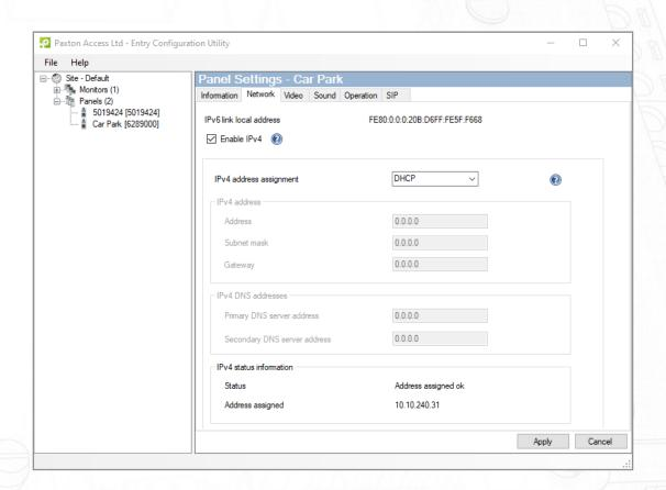
The SIP server uses IPv4 addressing for communication and so we need to obtain an IPv4 address for the panel.
