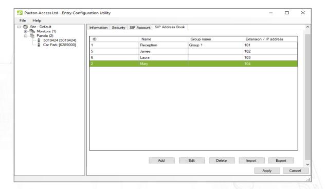
The two systems require a table to match each SIP client entry to a Entry monitor ID.
