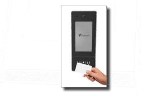
For PIN or code entry, touch the keypad icon , then enter your PIN or code. If a token is also required, presenting the token will open the keypad for you.
