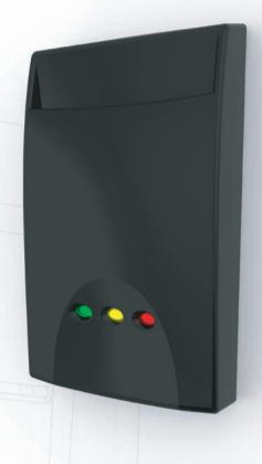
Our Proximity energy saving reader minimises energy wastage and saves customers money on their utility bills. The reader cover is designed to retain a user card. Once inserted, the card's presence in the reader toggles a relay that switches on all connected equipment. When the card is removed, the relay toggles back, turning all equipment off.
