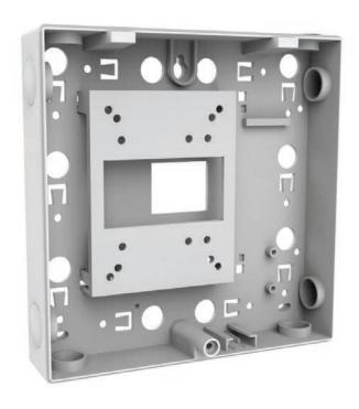
The single plastic housing is available for integration with a selection of different Paxton ACU's. A tamper switch is also installed which registers an alarm if the lid is opened when connected to an ACU. If integrating a Switch2 within the plastic housing, the 12V 1A PSU can also be fitted inside the enclosure to power the Switch2 control unit.
