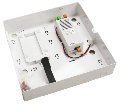
The 12/24V 2A AC/DC Power supply unit is available in either a plastic or metal cabinet. The cabinet can house both the 12/24V 2A AC/DC PSU and a Net2 ACU with the option to accomodate a 12V/7Ah back up battery if desired. A tamper switch is also installed which registers an alarm if the lid is opened when connected to an ACU. Please note that the Net2 nano ACU is not available for integration within the metal cabinet.
