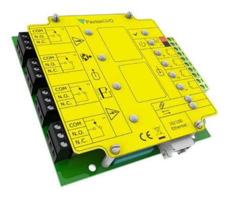
The Net2 I/O board is simple, yet powerful addition to the Net2 system. It can be wired alongside a Net2 door controller, to switch power on and off to electrical equipment to save money and energy. The board can control lighting, heating, water and air conditionoing by using the triggers and actions application in the Net2 software. These actions can be programmed for a particular time, or in response to a specific Net2 event.
