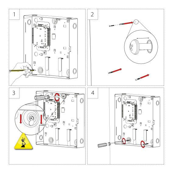
Note: This mounting process applies to all types of cabinet and housing regardless of size, material or power supply included.
