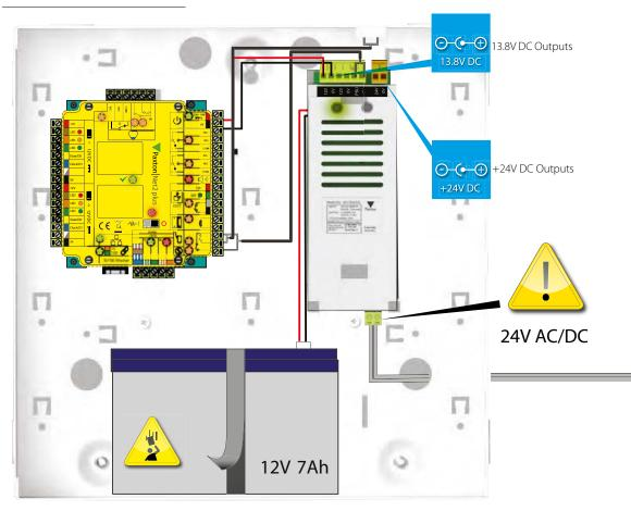
Note: Must be powered by a UL 294 Listed, Power supply or UL 603 Listed, power limited, power supply capable of supplying 24VDC, 2.3 A.
