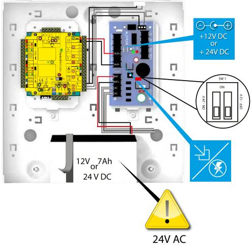
Note: Must be powered by a UL 294 Listed, Power limited, Power supply or UL 603 Listed, Power limited, Power supply capable of supplying 24V AC, 40 VA.
