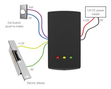
12V DC release current rating must be less than 1A.
