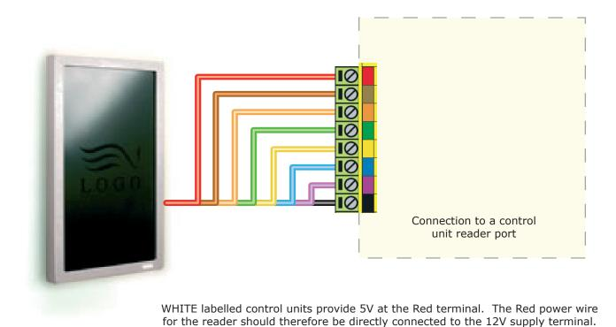
IMPORTANT: This reader cannot be connected in parallel with other readers and keypads.
