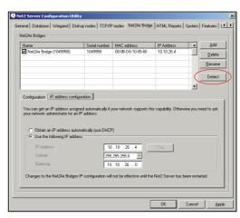
Only ONE Net2Air USB bridge may be used per system. Multiple Net2Air Ethernet bridges may also be configured.
