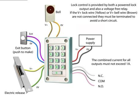
When using the relay output, it is not recommended to use the 'Lock wire setting' in the 'fail open' mode.
