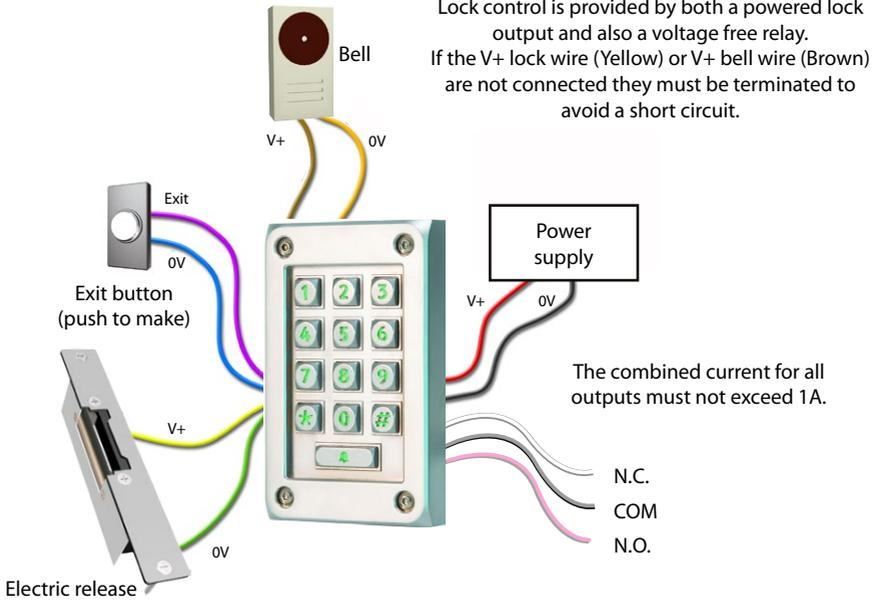
When using the relay output, it is not recommended to use the 'Lock wire setting' in the 'fail open' mode.
