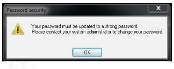
NOTE: The default operator account, 'System Engineer' is unaffected by this rule so access to the system can still be achieved in the event that this service is enabled, but the default 'System Engineer' operator account has not been updated to meet the requirement.
