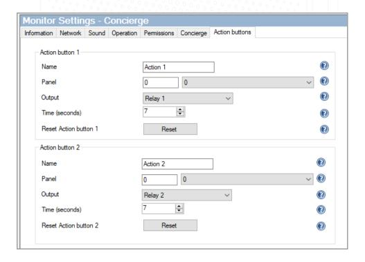
Enter a name for the action buttons, recommended to name them appropriately for the device they will trigger. This name will appear on the screen for the Premium monitor.
