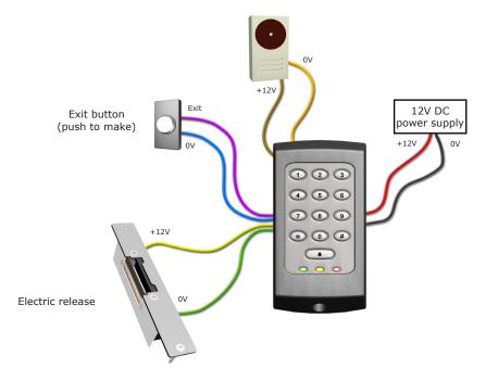
12V DC release current rating must be less than 1A.
