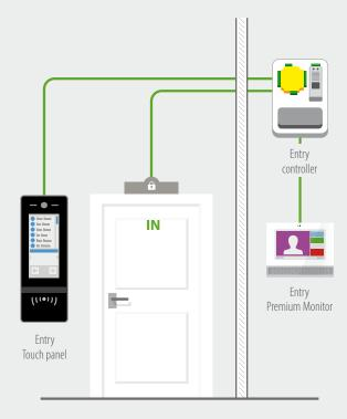
Standalone Entry system does not require connection to a network or server
