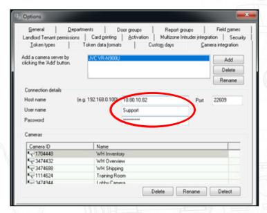
Enter the Host name. This will be the URL or IP Address of the DVR/NVR (digital video recorder/ network video recorder) server, you can also include a port number if this is required.
