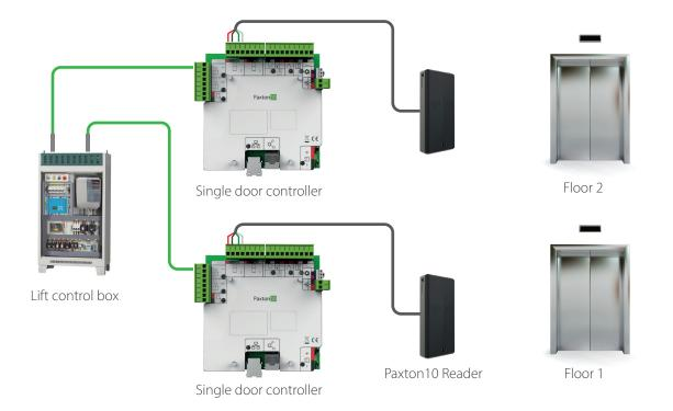
Alternatively, for a more cost-effective solution, one Paxton10 controller for every two lift floors may be used. This approach requires custom mapping in Paxton10.
