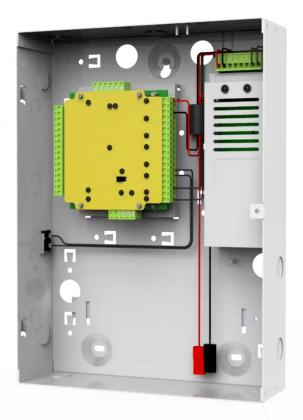
The 12V 2A Power supply unit is available in either a plastic or metal cabinet. The cabinet can house both the 12V 2A PSU and a Net2 or I/O ACU with the option to accomodate a 12V/7Ah back up battery if desired. A tamper switch is also installed which registers an alarm if the lid is opened when connected to an ACU or I/O board. Please note that the Net2 nano ACU and I/O board are not available for integration within the metal cabinet.
