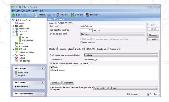
Net2 can also be configured to automatically produce a roll call report when the fire alarm input is activated. To enable this function, the Area for which the roll call report is to be produced must be selected from the drop down list at the bottom of the screen.
