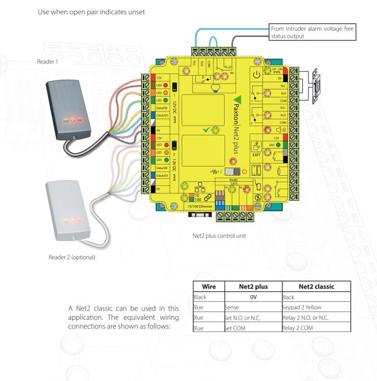
If the door on the ACU is normaly held open with a timezone, the ACU will not unlock the door until the intruder alarm has been unset.
