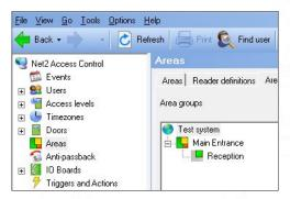
The two ACU's need to be linked as an Area Group. Both are using the Reader 1 (In) port and so the direction (Goes from - Goes to) needs be correct in the definition screen.
