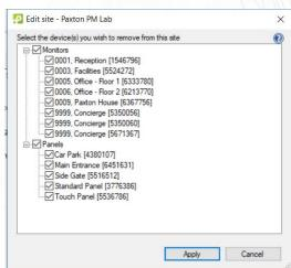
Devices can be grouped under a site name that is secured with an engineers code for that site. This means you can install multiple panels and monitors on one network but have certain panels that only connect to specified monitors. The individual site can then be selected when logging in.
