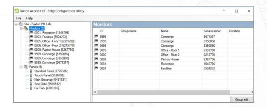
Click on the Monitors folder to expand the list into a tree view. Individual monitors can then be selected from that list. Multiple devices can be edited by using the Group edit function.
