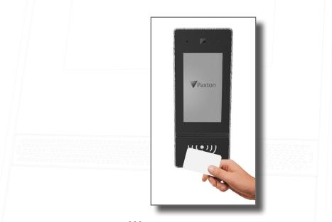
For PIN or code entry, touch the keypad icon ••• , then enter your PIN or code. If a token is also required, presenting the token will open the keypad for you.
