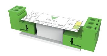
Compact systems use a 12V DC switched voltage to provide an output for a lock. This is not suitable in situations where volt free contacts are required for controlling external equipment, such as roller shutters or 24v locks. The compact relay module has been designed to be connected across this output (Green / Yellow wires) and provide switched (NO / NC) volt free contacts.
