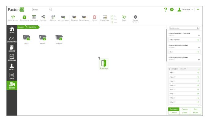
Once a component from the Paxton10 controller is mapped to a device in Paxton10, the controller is then bound to that Paxton10 system, and can't be detected or controlled by any other system.
