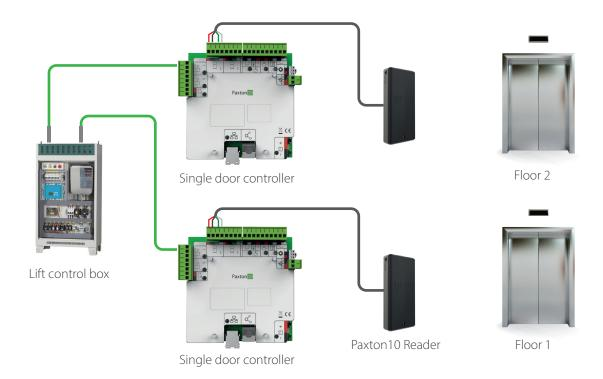
Alternatively, for a more cost-effective solution, one Paxton10 controller for every two lift floors may be used. This approach requires custom mapping in Paxton10.
