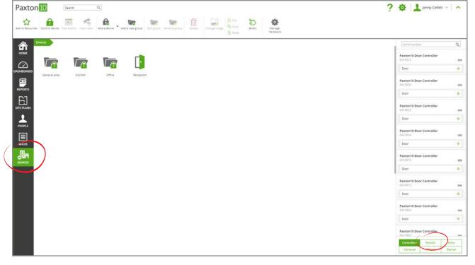
4. Click on the move icon under the PaxLock Pro you wish to add to your system and drop it onto an empty space to create a new device in Paxton10, or drop it onto an existing 'PaxLock Door' device to map the PaxLock Pro to the device
