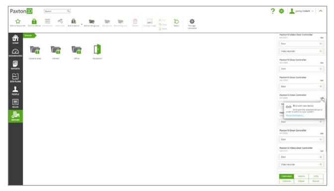
Note: When first binding a PaxLock Pro to a Paxton10 system, there will be a 10 minute time period for the unit to update. The status of the PaxLock Pro can be viewed in Manage Hardware.
