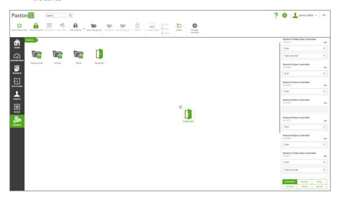
Once the PaxLock Pro is mapped to a device in Paxton10, the PaxLock Pro is then bound to that Paxton10 system, and can't be detected or controlled by any other system.
